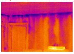
Infrared thermal imaging is utilized with blower door depressurization techniques to determine the quality and performance of your building enclosure.
